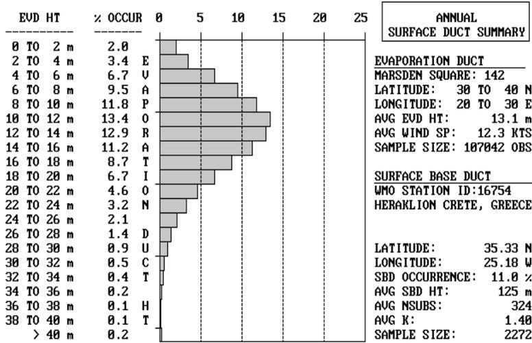
Figure 3-20: Evaporation Duct Histogram for Marsden Square 142.
