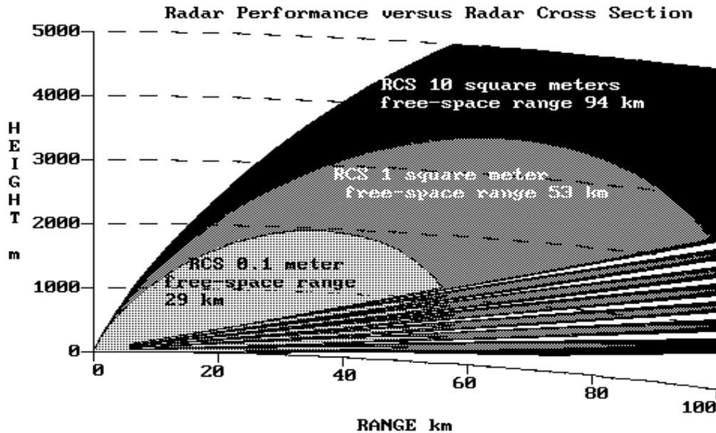
Figure 3-5: Comparing Radar Cross-section Effects.
