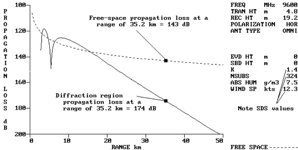
Figure 3-21: PROPR Display for Standard Atmospheric Conditions.
