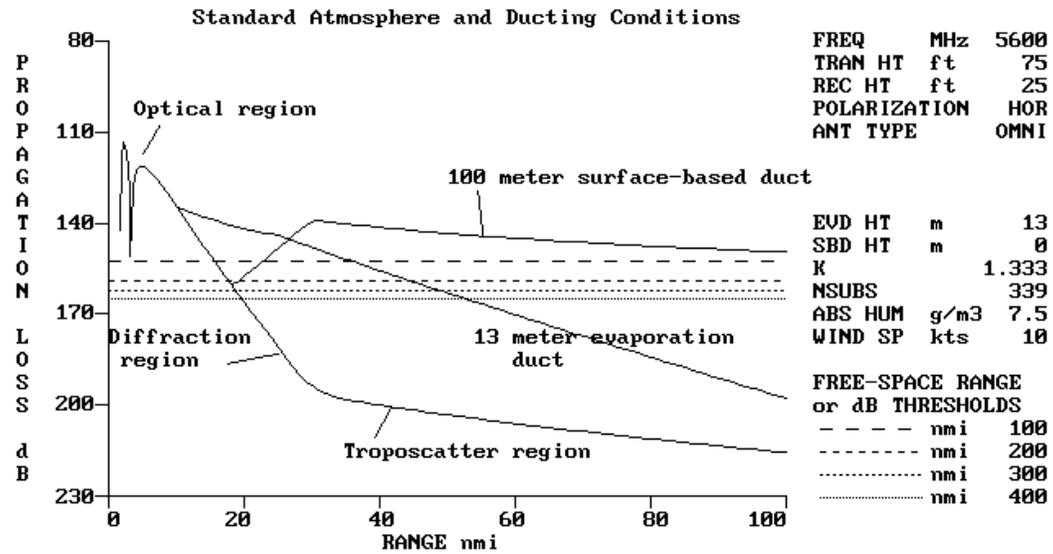
Figure 3-9: PROPR - Comparing Ducting and Standard Atmosphere Effects.
