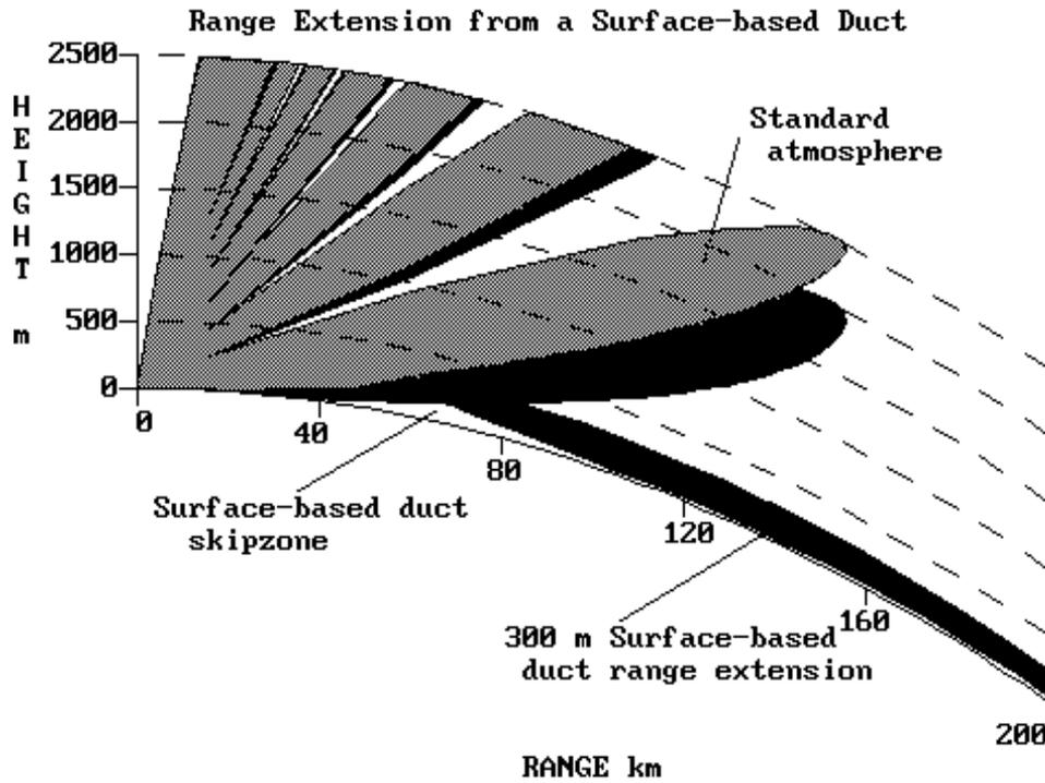
Figure 3-3: Comparing Ducting and Standard Atmosphere Effects.
