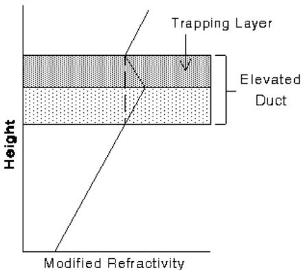
Figure 2-6: Elevated Duct.
