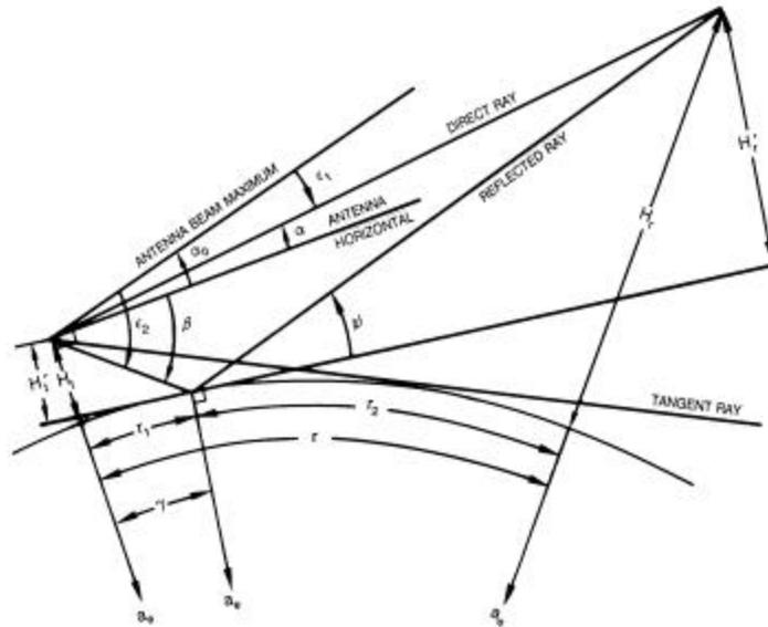
**Figure 6-1: Two path optical interference region.**
