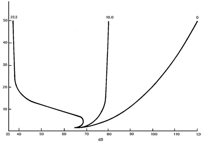
Figure 6-2: Evaporation Duct Height-Gain Curves displaying very little variation with height. The minimum scaled height used for calculating the height-gains is 1.0 meter and heights below this are set equal to this value.
