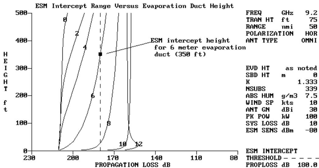
Figure 3-13: PROPR - Parametric Study in Evaporation Duct Height.
