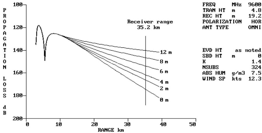
Figure 3-23: PROPR Display for Various Evaporation Duct Heights.
