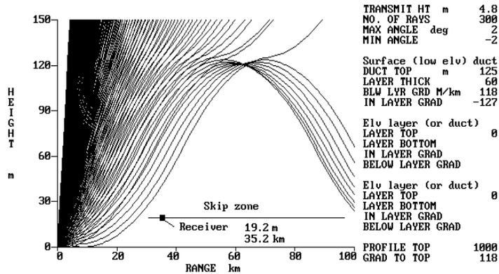
Figure 3-22: RAYS Display for Surface-based Duct Conditions.
