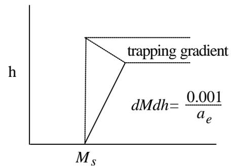
Figure 6-5: Surface-based Duct Model
