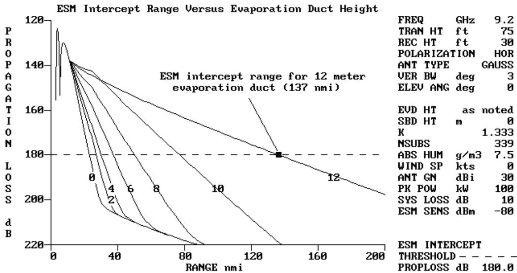
Figure 3-12: PROPR - Parametric Study in Evaporation Duct Height.
