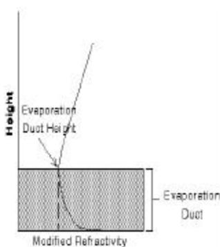
Figure 2-5: Evaporation Duct.
