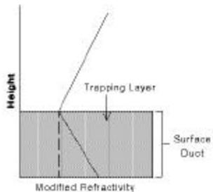
Figure 2-3: Surface duct.
