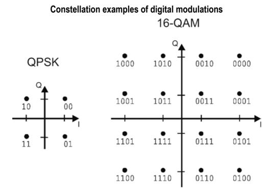
Representation of the constellation of possible positions of the carrier in the phase (angle) / amplitude (distance from the center), for QPSK and 16QAM modulation schemes. The numbers near each point of possible positioning of the carrier, indicate the transmitted Transport Stream bit sequence when the carrier has that position.
