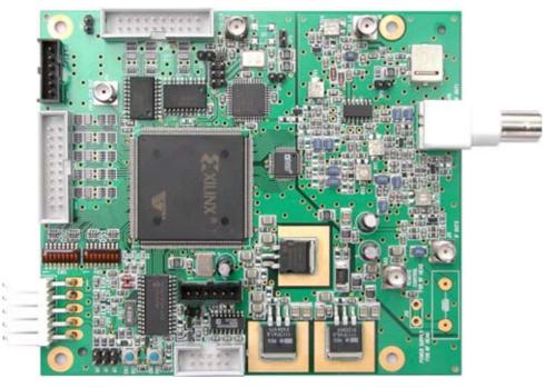
Figure 2 QPSK (DVB-S) and QAM (DVB-C) Modulator board - (ABE production)
