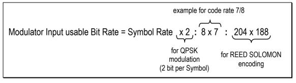
the difference is in the signal to noise/disturbances ratio: for example, with a 1/2 Code Rate the signal margin is around 4dB higher than using a 7/8 Code Rate, but the useful data bit rate is lower.
