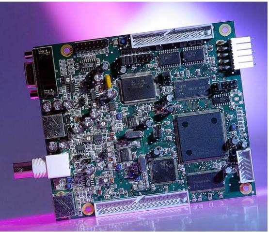
Figure 1 - MPEG-2 encoder board (ABE production)
